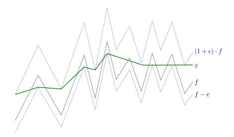
Figure 1: This figure illustrates the described model. A piecewise linear function f with n = 14 sampling points is plotted. This function is approximated given a relative upper error bound  $\epsilon$  and an absolute lower error e. The resultant function g has m = 8 sampling points.
