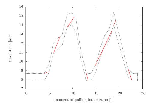
Figure 7: This figure illustrates the result of Algorithm 3. We approximate a piecewise linear function with 125 sampling points taken from our application and plot the tunnel (dashed) with the determined windows. The lower border of the tunnel is the given function which defines the travel-time for a certain street section dependent from the moment of pulling into this section.
