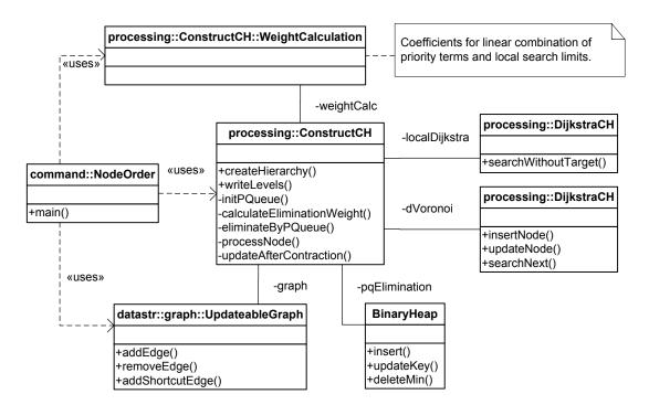
Figure 33: An UML class diagram for the use case: node order selection.
