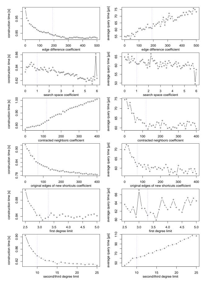
Figure 28: Sensitivity analysis with road network of South Carolina (USA). Parameters used: edge difference multiplier 190, search space multiplier 1, contracted neighbors multiplier 120, original edges term multiplier 70, hop@degree limits: 1@3.3, 2@10, 3@10, 5 46
