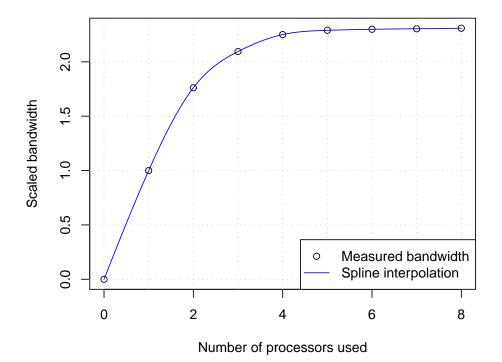
Figure 5.2.: Different models for memory bandwidth on the Xeon system.
