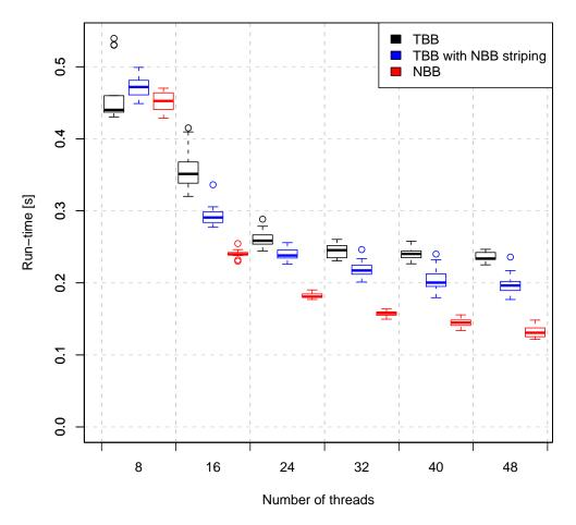
Figure 4.2.: Run-time comparison of query 21 on our Opteron system with TBB and NBB.
