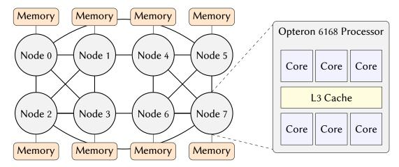
Figure 2.2.: Schematic view of our Opteron system.
