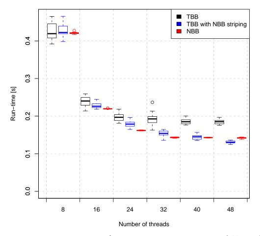
Figure 4.1.: Run-time comparison of query 5 on our Opteron system with TBB and NBB.
