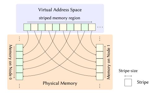
Figure 3.2.: Striping memory over two nodes.
