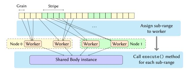
Figure 3.6.: Iterating over a striped memory region.
