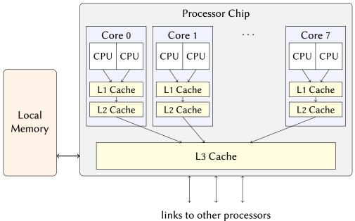
Figure 2.1.: Cache hierarchy of Xeon processors, using the X7560 model as example.
