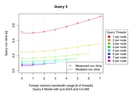
Figure 5.4.: Measured and modeled run-time of query 5 on the Xeon system.
