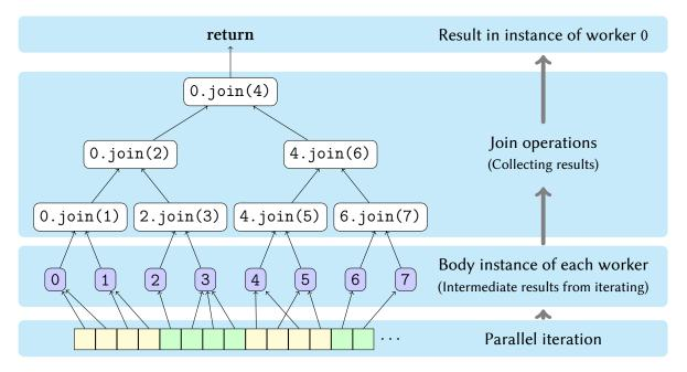
Figure 3.7.: Reduction of parallel\_reduce body instances.
