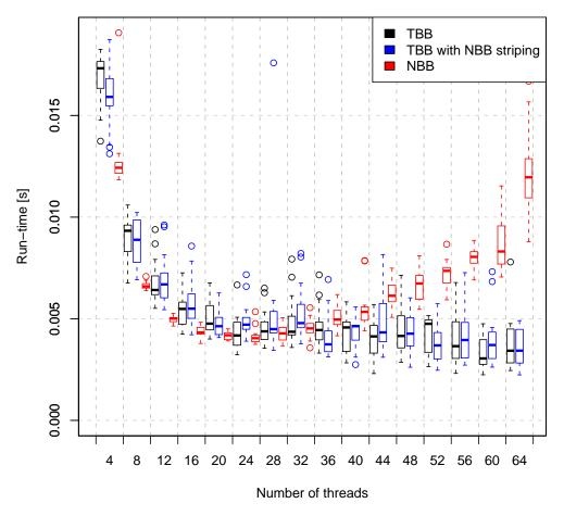
Figure 4.6.: Run-time comparison of short-running Query 17 on our Xeon system.
