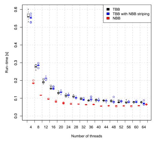
Figure 4.4.: Run-time comparison of query 13 on our Xeon system with TBB and NBB.
