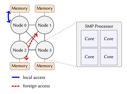
Figure 1.1.: Schematic view of a NUMA system consisting of SMP processors.
