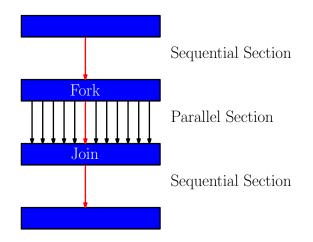
Figure 1: OpenMP Utilizes a Fork/Join Model
