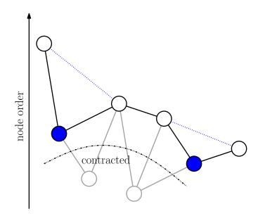
Figure 2: An example of an independent node set. The filled nodes are independent of every non-contracted node.
