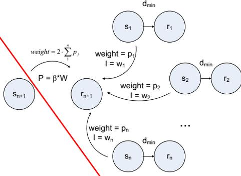
**Figure 2: Reduction from Knapsack: the weight of simultaneously scheduled links is maximized if and only if the sum of the values  $p_j$  assigned to them is maximized and the knapsack capacity  $W$  is not violated.**
