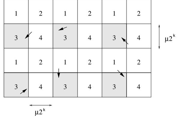
**Figure 3:** In line 7 of Algorithm 1, the algorithm picks all squares numbered by  $j$ . The example shows an inner loop iteration for length class  $R_k$  and  $j = 3$ . The algorithm schedules one unscheduled link from each selected square (if there exists one).
