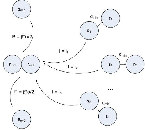
Figure 1: Reduction from Partition: link  $l_{n+1}$  (or  $l_{n+2}$ ) can be scheduled if and only if the interference caused by simultaneously scheduled links  $s_j, j \in \{1 \dots n\}$  is less or equal to  $\sigma/2$ .
