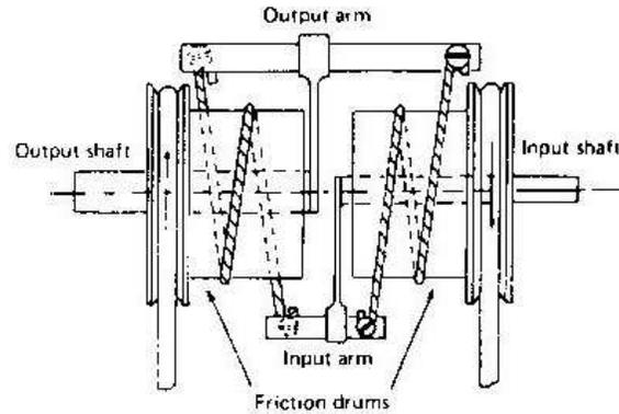
Figure 2: Principle of Bush's torque amplifier (from the 1931 article by Bush, taken from [Wil00])
