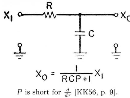
Figure 4: An electrical integrator [KK56, p. 13]
