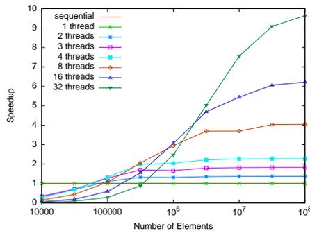
**Fig. 5.** Computing partial sums of 32-bit integers.
