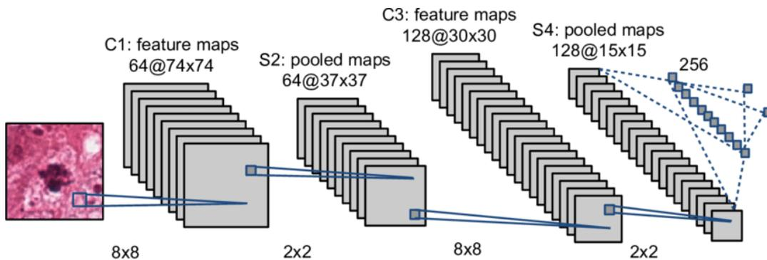
Figure 2.3: Example of a CNN architecture [29].
