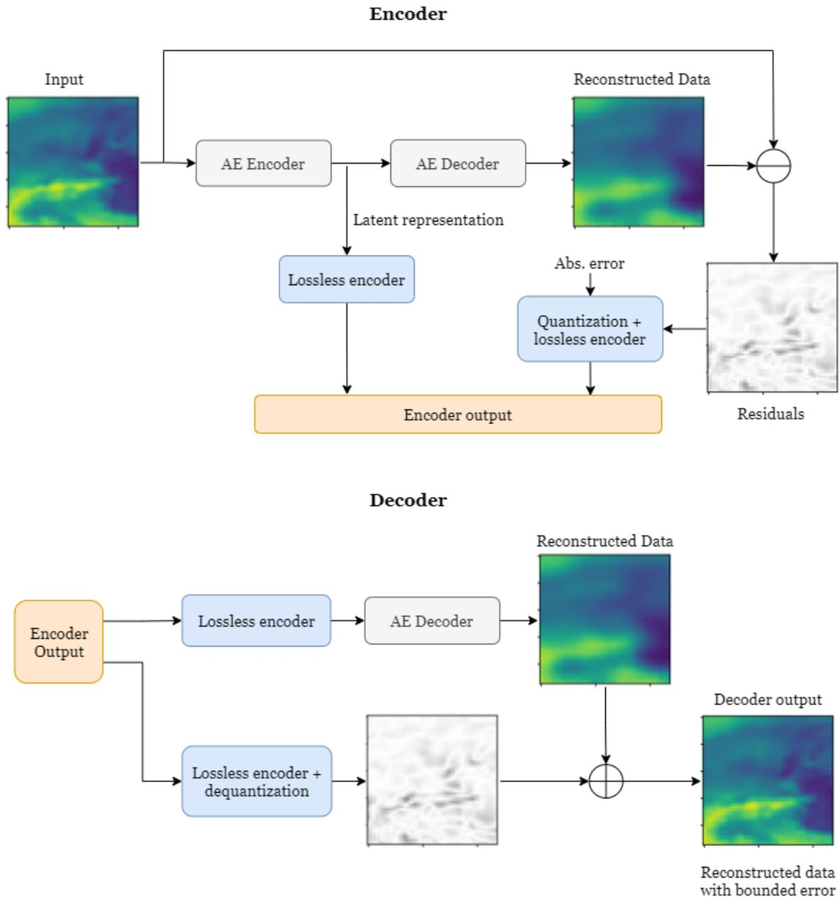
Figure 4.1: *Compression algorithm architecture.*
