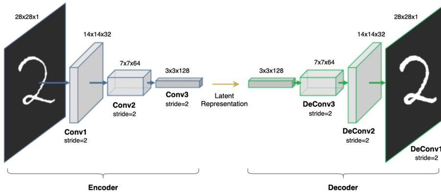
Figure 2.5: Example of a convolutional autoencoder. Adapted from [34].
