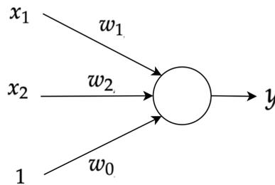
Figure 2.1: *Perceptron with two inputs and one output.*
