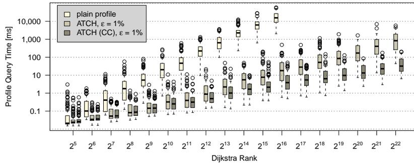
**Fig. 1.** Profile query times over the Dijkstra rank for different methods. CC means corridor contraction is used, otherwise a profile search in the corridor is performed.
